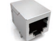
DG1128-01 Series PCB Jack 8 Positions W/ Full Shell 3.05mm Type
